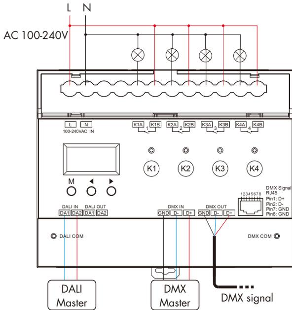
**Note:** The maximum surge current of the AC output is 120A, the sum of surge current of multiple resistive load or inductive load (LED drivers) should not exceed its maximum value. Otherwise, the product will be overloaded and damaged.
